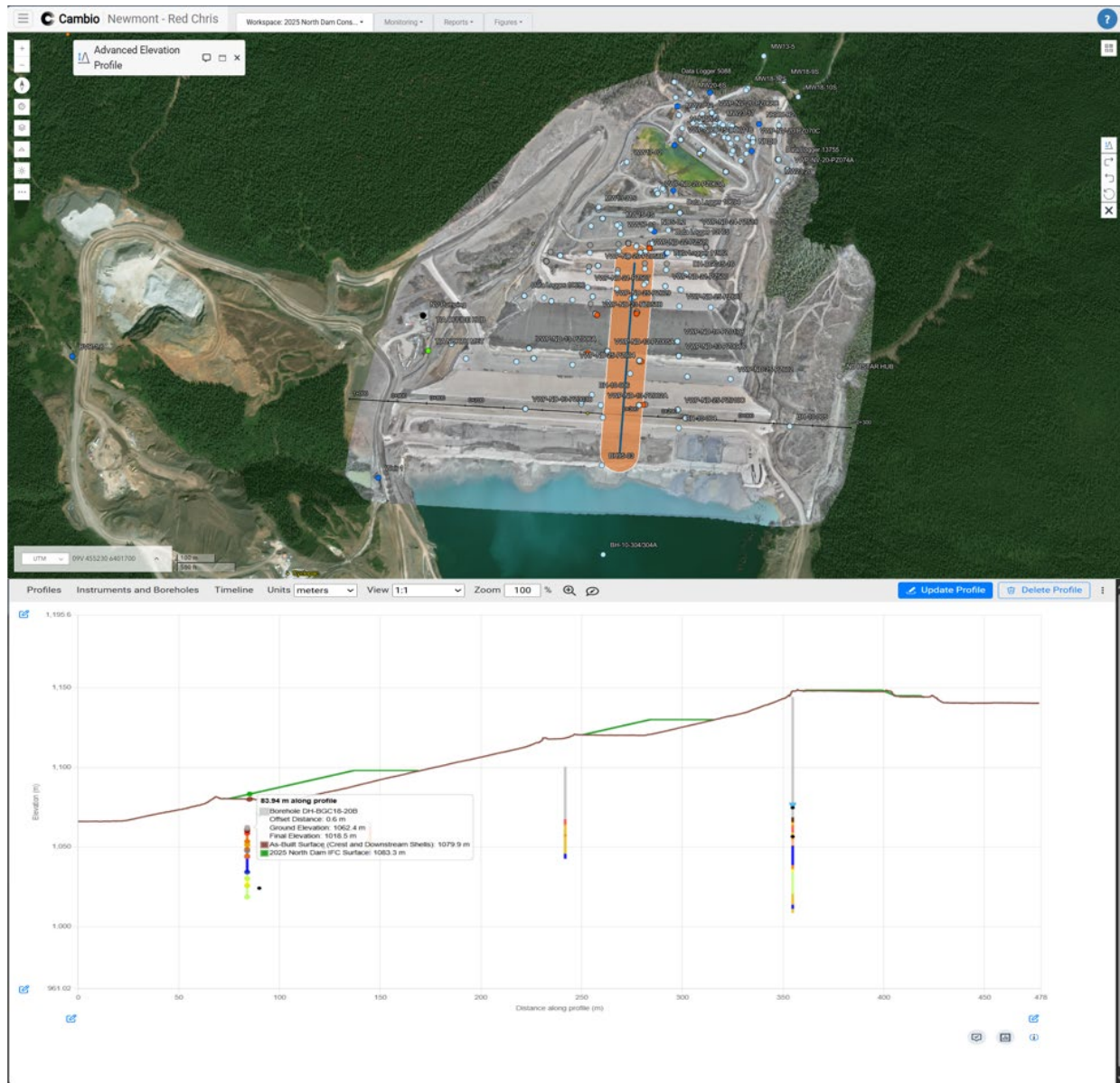
Figure 5: User-generated plan and section views of the North Dam showing borehole locations, instrument installation depth, latest readings, and stratigraphic stick-logs
