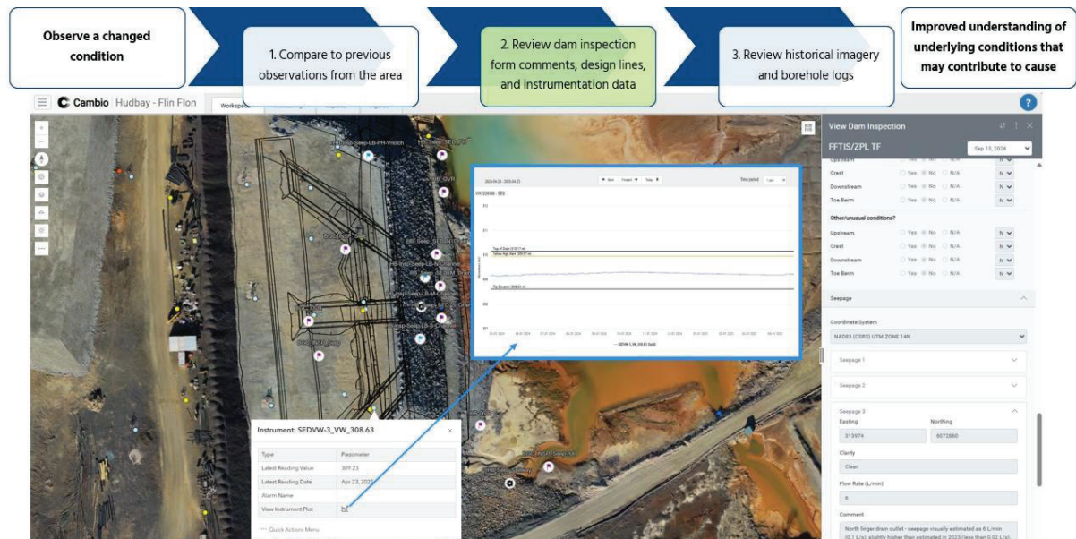
Figure 2 A view of the Cambio web platform showing a dam inspection form, Observation Points, instruments, and design lines
