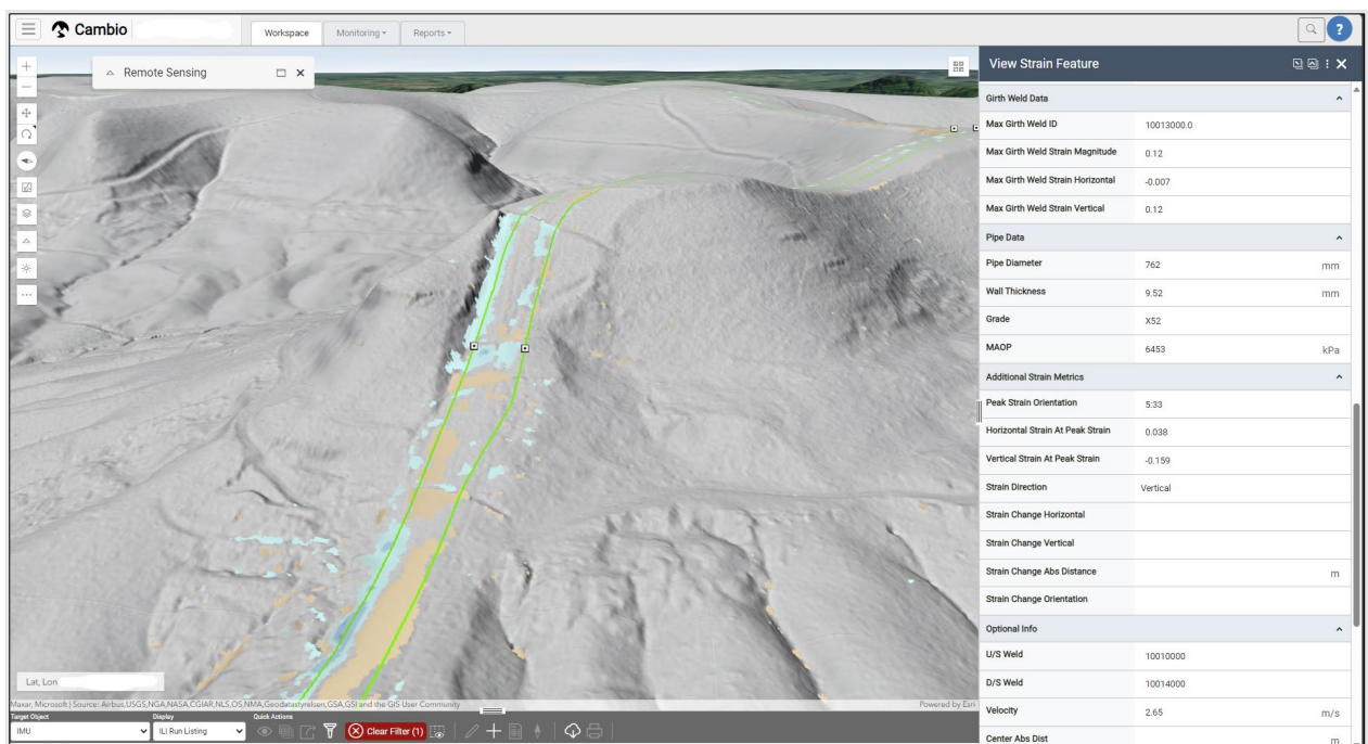
Figure 6. Example demonstrating the capability to simultaneously observe strain feature data and change detection results, enhancing comprehension of potential hazards at a site.
